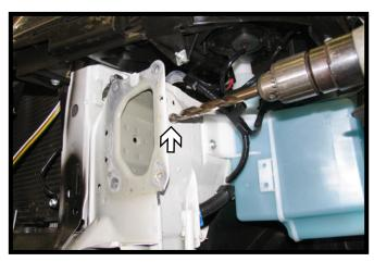
9. Using a 17/32" drill bit, ream the existing hole in the frame as shown. Do this on both sides of the vehicle.
