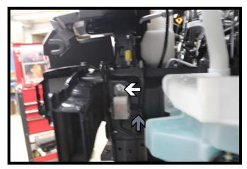
4. On the driver side, using a 10MM socket, remove the bolt from the sensor bracket. Remove the wiring clip and move the sensor and wiring out of the way (gray).
