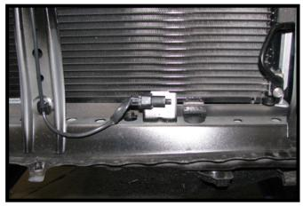
8. Bend the temperature sensor bracket inwards toward the radiator.
