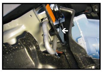
14. On the bottom baseplate hole, insert the spacer tube between the frame and the baseplate. Insert a 3/8"-16 x 2" bolt, 3/8" flat & lock washer and 3/8" lock nut. Do this on both sides of the vehicle.
