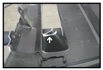
Hold the fascia as close to it's original position and mark the backside of the fascia, trim as needed. Reinstall the fascia.
